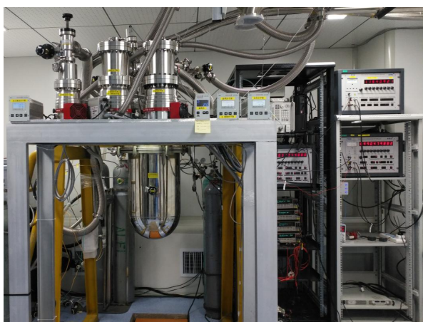
Figure 2. Left: Single Pressure Refractive Index Gas Thermometry at TIPC-CAS in China. Right: Total uncertainties ( k=1 ) for thermodynamic temperatures T_{\text{SPRIGT}} from 5 K to 24.5561 K.
