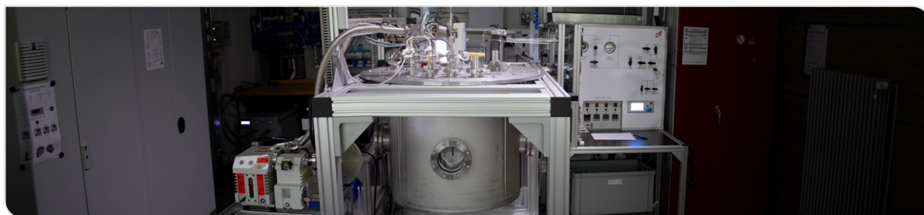
Figure 1: The Cryogenic Phase Equilibria Test Stand CryoPHAEQTS.
